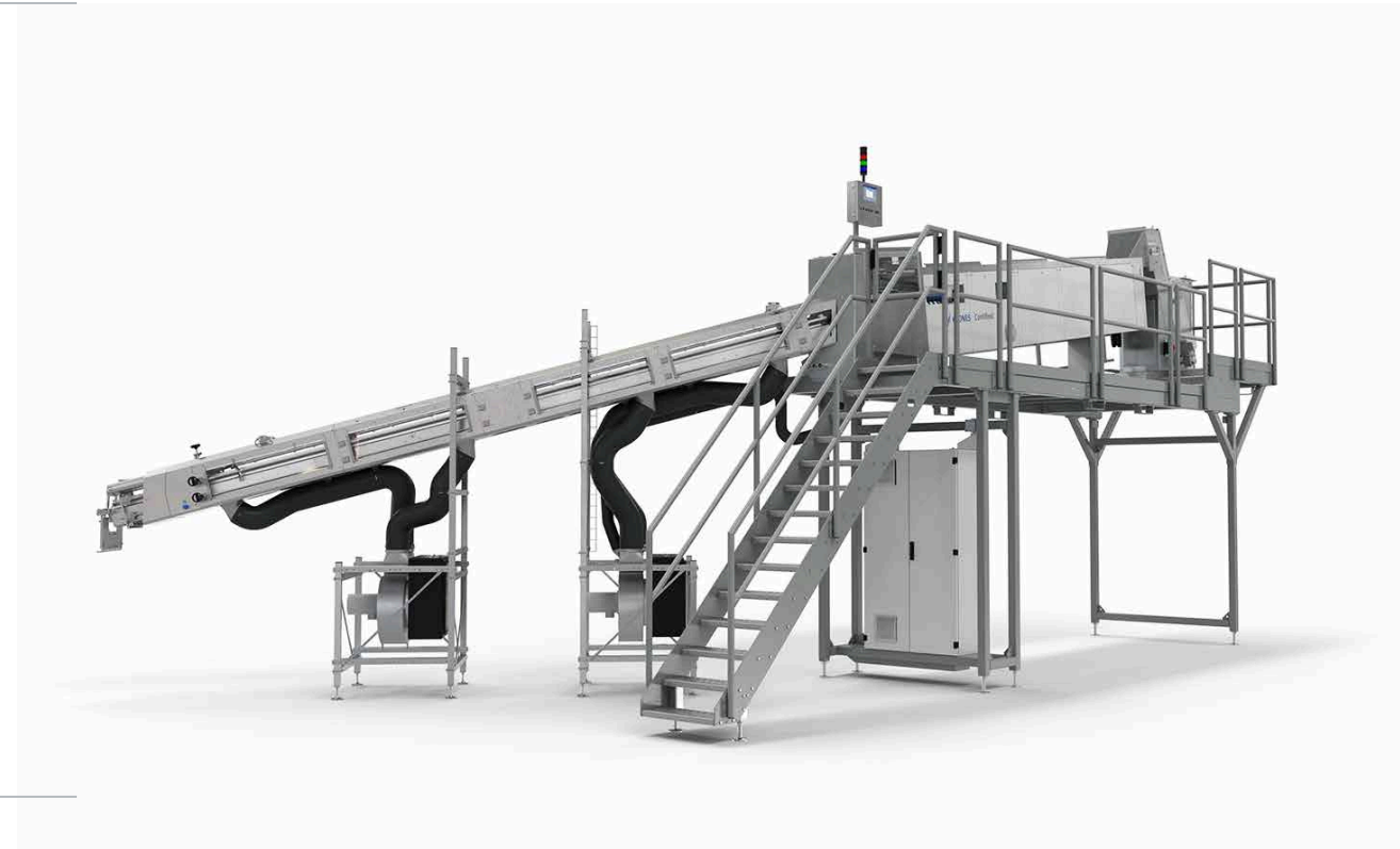
Contifeed with air-assisted feed rail
