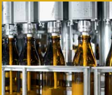
Viscofill uses a piston to actively feed product in a two-step process: The piston draws the correct quantity of product into the dosing cylinder on the upstroke and then pushes the product out to the container on the downstroke.
