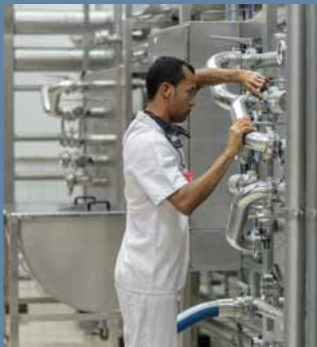
A CIP system with eleven different tanks provides automatic cleaning of the entire cold end.
