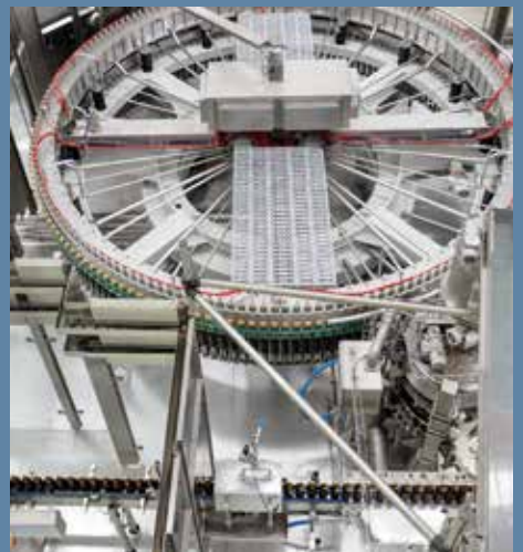
Mecafill VKP-V filler with 176 filling valves
