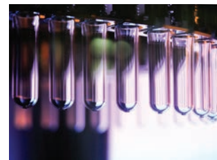
The Contiform (sc) can produce up to 81,000 containers per hour with a volume of up to 0.75 litres.
