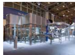
KRONES has synchronised a stretch blow moulder, labeller, and filler in the new ErgoBloc L.
