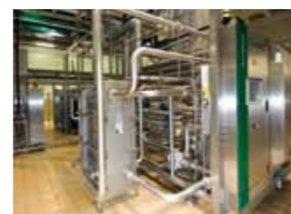
VarioFlash B is KRONES' new flash pasteurisation system.
