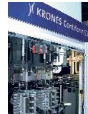
The speed-enhanced Contiform S series of stretch blow-moulders manufacture up to 44,800 PET bottles per hour at high speed and using the highest possible level of technology. This corresponds to more than 14 bottles per second.
