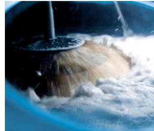
The Stromboli wort boiling system makes it possible to bring total evaporation in the wort boiling process down to a low level and thus achieve a high level of energy efficiency in the brewing process.
