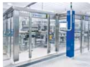
The filler's modular design makes it easy to synchronise into a bloc arrangement with other machines.
